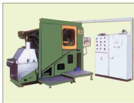
100 Bar High Pressure Die Casting machine from HADI GMBH, Austria costing Rs. 2.5 crores
